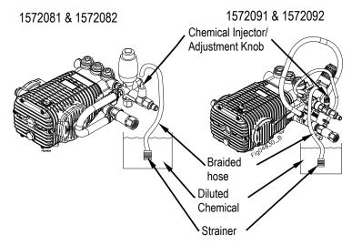
**Note:** Adding accessories (IE: telescoping wands, extra length of High pressure hose, Non factory triggers) will affect chemical injector performance or cause it not to operate at all.
